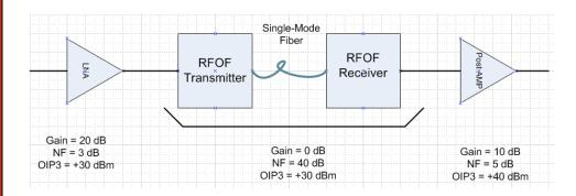
1/(OIP3End-End) = 1/(OIP3LNA\*GRFoF\*GPA) + 1/(OIP3RFoF\*GPA) + 1/(OIP3PA) 1/(OIP3End-End) = 1/(1000\*1\*10) + 1/(1000\*10) + 1/10000 = 1E-4 + 1E-4 + 1E-41/(OIP3End-End) = 3.33E3 OR +35.22 dBm
