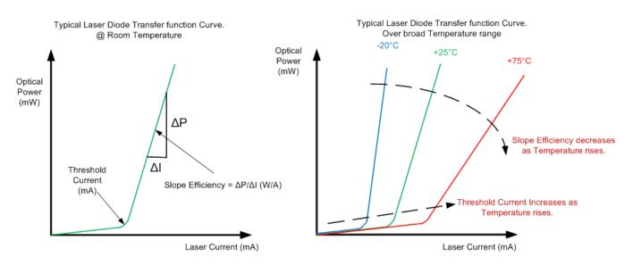
In Case of Cooled DFB Laser Transmitter, the slope Efficiency of the laser is not changed even though the Transmitter module will be exposed to wide temperature variations of up to -40C to +85C
